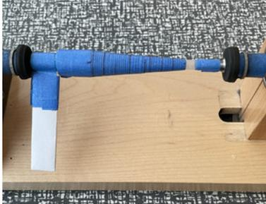
1. Mount your winding device\* on a double-ended bobbin winder.
