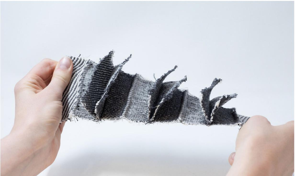
Sample 1 is the first Jacquard-woven fabric made during this residency. It combines self-folding techniques with partial weft passes, which are a unique capability of hand-operated Jacquard looms.
