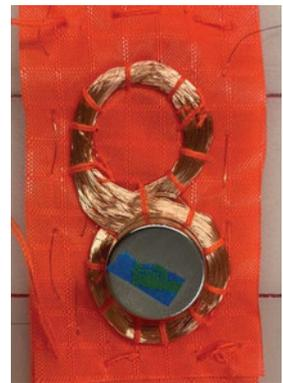
An assembly of two figure-eight coils (only the top one is visible). The two sides of the figure eight have opposite polarity. The magnet is drawn to a distinct point on the assembly for each combination of the two coils' polarities.
