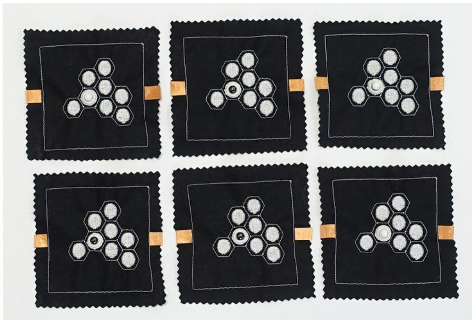
*1-Bit Textile*, a swatch created by Posch and Kurbak that occupies two distinct states (magnetic bead facing up or down) depending on the polarity provided to an electromagnetic coil.
