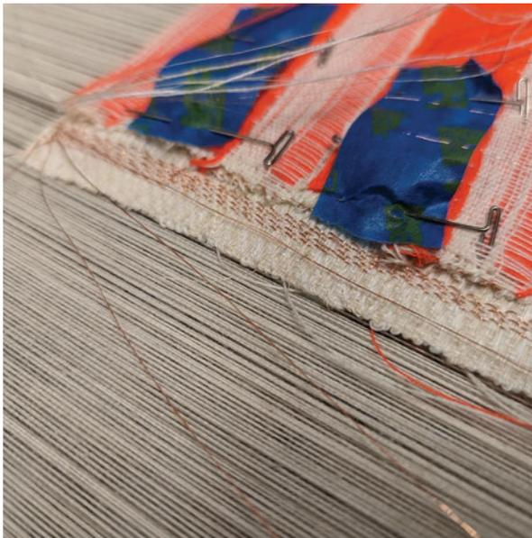
Routing the magnet wire was not explicitly defined in the weave draft. We used the existing twill structure as a guide for when to bind the wire to the fabric.
