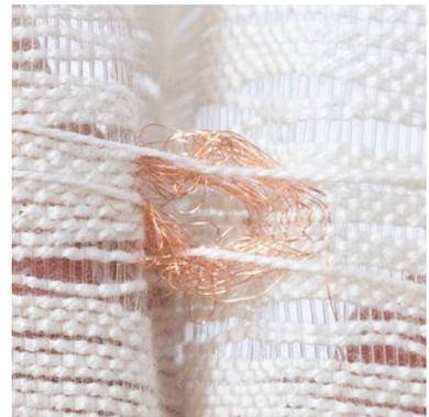
Simple helical or spiral coils create push-and-pull actuation; arrays of multiple coils can create side-to-side sliding actuation when powered in a specific sequence. Ferrous metal cores increase the strength of cylindrical electromagnets but had no effect on our flat versions. Handmade coils inevitably have overlaps where successive wire wraps cross each other, diminishing the strength of the magnetic field.
