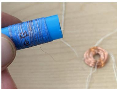
16. Where the coil is still connected to the spool of magnet wire, unspool about 24", cut and wrap around a bobbin.
