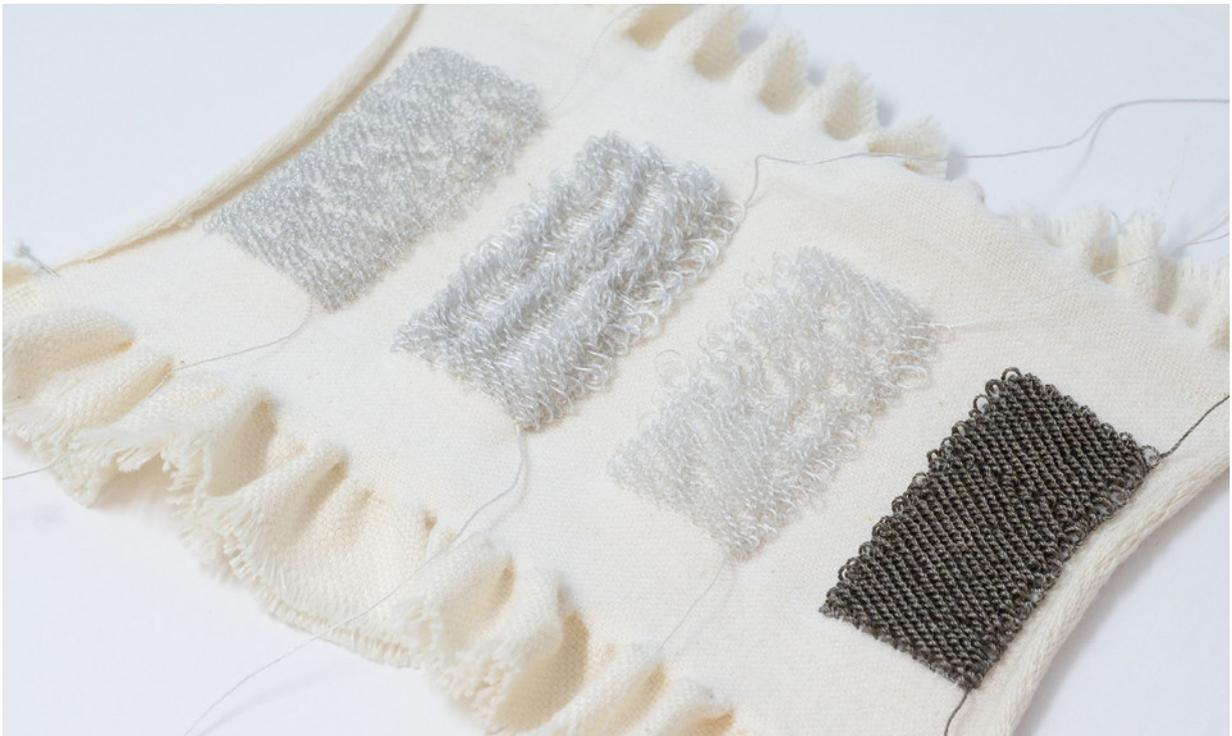
Sample 2f (top) and 2g (bottom). Sample 2f has a 1:1 ratio of conductive picks to base yarn picks, which proved to be too dense and rigid and prevented weft loops from forming when the fabric shrank horizontally.
