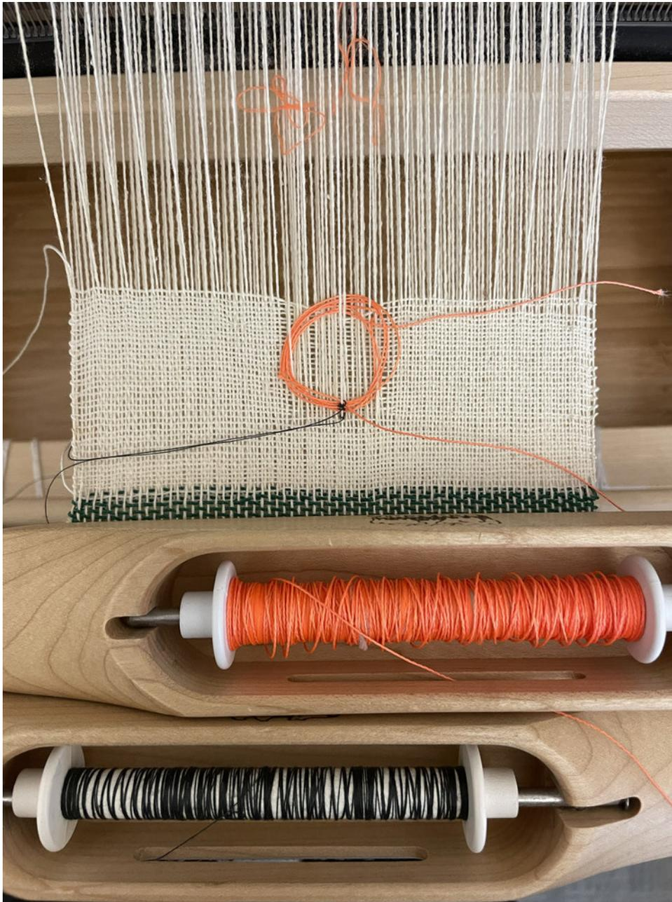
Prototype of a loom-controlled coil, with orange fishing line used as a stand-in for magnet wire. The darker weft yarn is a binding thread that keeps the bottom edge of the coil anchored to the base fabric. It must be tightened by hand because it is behind the fell line and cannot be beaten into place by the reed.
