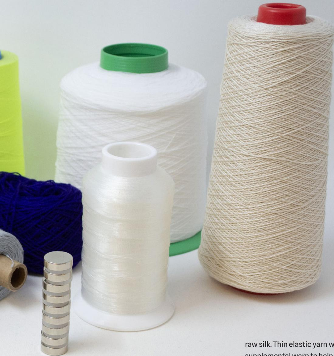
We initially used nylon monofilament combined with undyed cotton to lend stiffness to the fabric, but found it too rigid and a bit unwieldy to work with. Instead, we shifted toward a “kitchen-sink” weft with many yarns bundled together, eventually choosing a mix of bleached and unbleached linen, paper, and
