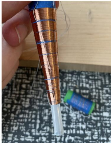
11. Remove the winding device from the bobbin winder.
