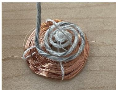
17. Twist all counting threads together and lower them onto the surface of the coil (they will naturally spiral) to keep them tidy and to mark the upper face of the coil.
