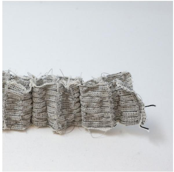
Sample 5 uses long weft floats interlinked with short warp floats to create a system of layers that can slide sideways relative to each other. Elastic floats give the layers an accordion-pleated and slightly crumpled look.
