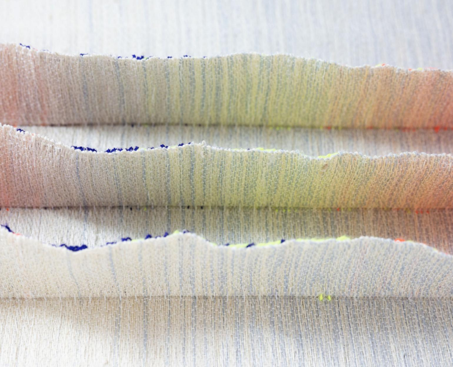
The next prototype tested mixing of multiple neon colors, which had to be done with a relatively coarse gradient stripe due to the constraints of shuttle passes in the existing file configuration. Still, the colors showed up as a diffuse blend due to the flaps' translucency and light-scattering abilities. This was also the first iteration in which magnets and coils were added on-loom, providing a very necessary dry run before Elizabeth wove the final piece.
