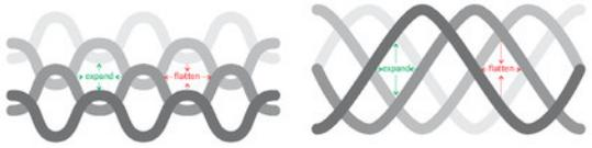
Two variations on 4-layer lattice structures inspired by 3D weaving “layer-to-layer” and “through-the-thickness” warp movements.
