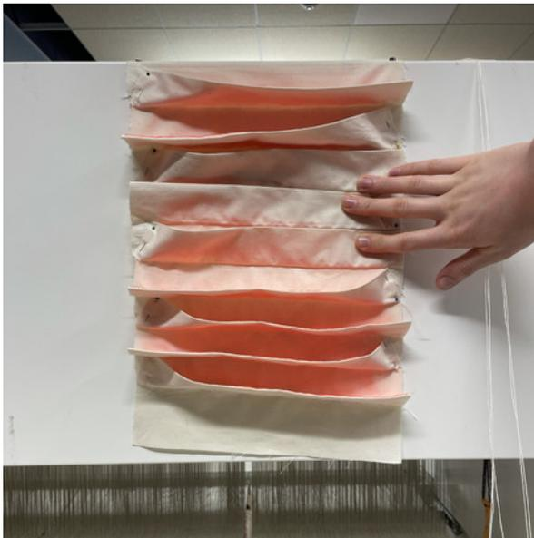
Second sewn prototype, with neon orange ripstop lining the interior of every flap.
