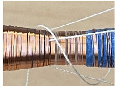
6. Wind 100 rotations, moving slowly from the start to the end of the first marked section. Wire wraps should be side by side, not overlapping.
