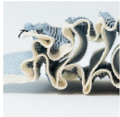
Sample 4b is a version of a spacer fabric with square cells and elastic floats at the corners. It uses a partial-weft technique to create parallel vertical walls between the upper and lower fabric layers.
