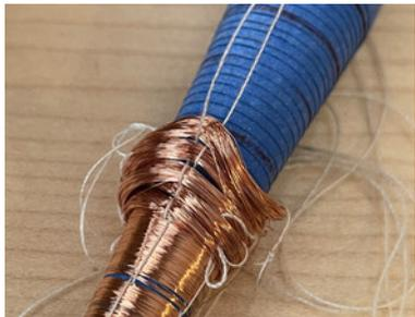
13. Pull both ends of each counting thread to tighten the slack running through the coil.
