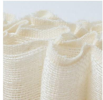
Sample 7d is another four-layer design with offset joining points between layers and a heavy-duty polyester weft.
