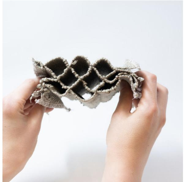
Sample 0 was the very first fabric woven during the residency, on an 8-shaft table loom. Similar to sample 7b, there are 4 layers joined at regular intervals to form a lattice, but in this fabric, both warps and wefts exchange positions at each joining point, creating the appearance of multiple fabric planes intersecting.
