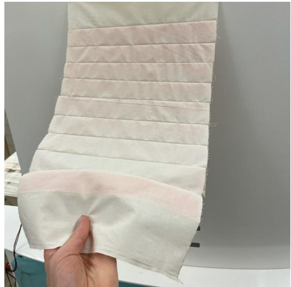
Reverse side of the second prototype. The base fabric is translucent and shifts in hue when neon strips are near.
