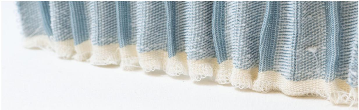
Sample 7a resulted in smaller peaks and valleys due to internal elastic floats joining layers together more often.
