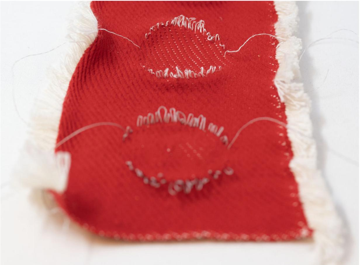
Sample 2e (top) and 3a (bottom) use a crimped nylon yarn that shrinks up to 50% when steamed, causing the surrounding non-shrinking yarns to buckle and form compressible loops.
