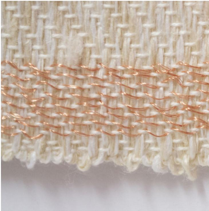
Magnet wires weave into the cloth structure towards a single connection point on the back of the cloth.
