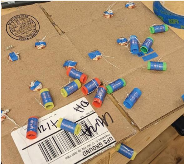
Preparing 16 800-turn coils, with labeled and color-coded bobbins to ensure they could be correctly identified when wiring the final piece.
