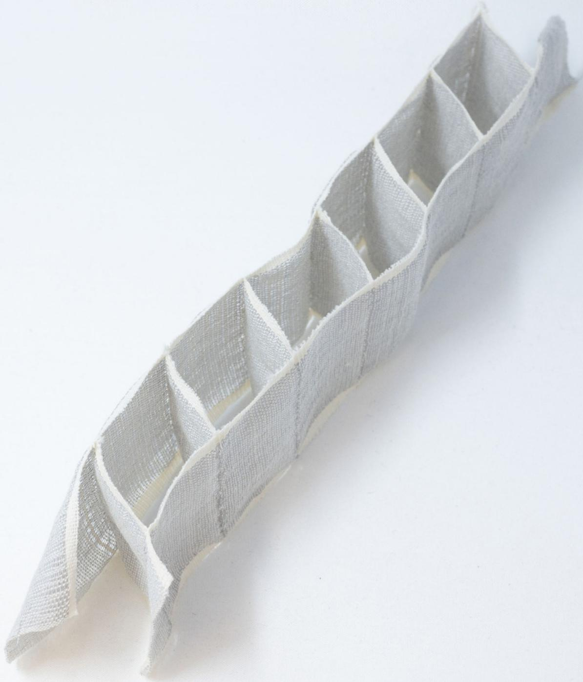
Sample 4a is a lightweight, crisp square-cell spacer fabric made with partial weft passes in a single material: bonded nylon thread. It was woven flat on the loom and its cells have a tendency to collapse to their original state.
